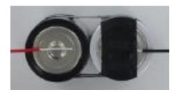
5. The pack is now ready to provide power to your experiments. It is important that the bare wires do not touch each other and cause a short circuit. We recommend that you temporarily cover the end of these bare wires with electrical tape to avoid accidental shorting of the batteries.
